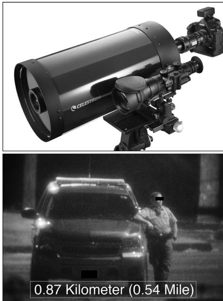
Figure 1-1a. Extreme distance photography during the day and at night is possible using appropriate equipment and technique. Upper image: Ultra-high-magnification night vision photography system. The night vision weapon sight serves as a finder scope, which is essential for the extreme distances the authors present in this book. Lower image: Using the electro-optical system in the upper image the surveillance specialist photographed this police officer from a distance of 0.87 kilometer (0.54 mile). Text discusses and illustrates this and other extreme-distance night vision photography methods.
